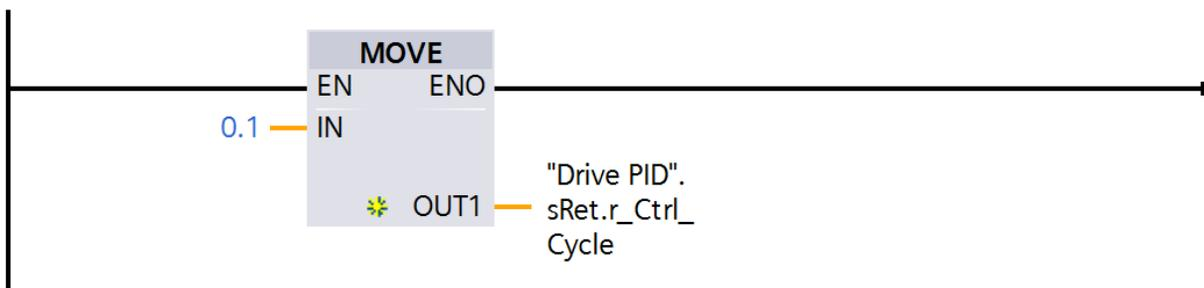
Network 5 : PID Block (Linear PID for Drives Output
